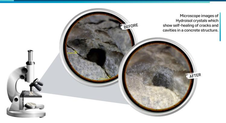
The formation of cracks or cavities in needle-headed form of crystalhydrate occurs gradually in concrete with HYDROISOL admixture.
